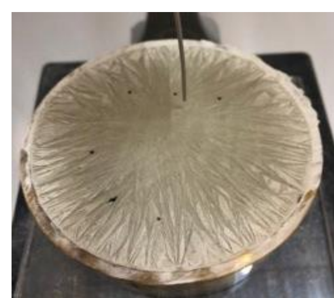
Frost appeared on paste sample at 0°F - Vicat Needle Penetration test
