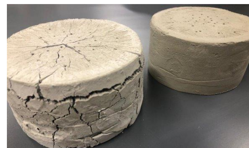
Cement pastes after Vicat Needle test - left sample is a couple days after test and the right sample is a few minutes after test at room temperature
