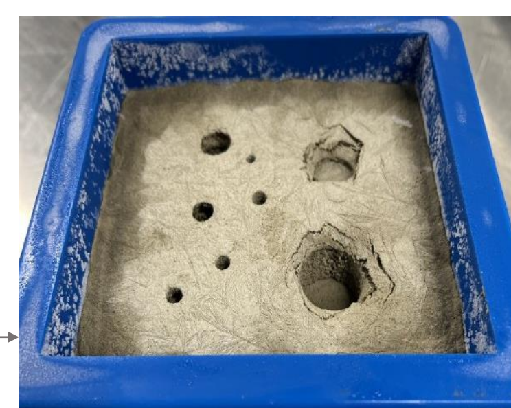
Cement pastes after Vicat Needle test - left sample is a couple days after test and the right sample is a few minutes after test at room temperature
