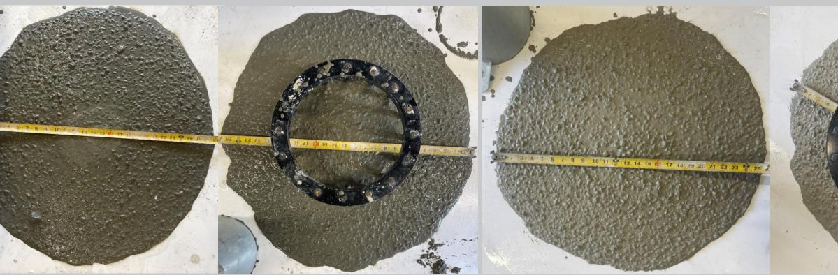
**PC-SCC w/c 0.37** 26.5 in. slump flow 26 in. J-ring passing ability 8% column segregation
