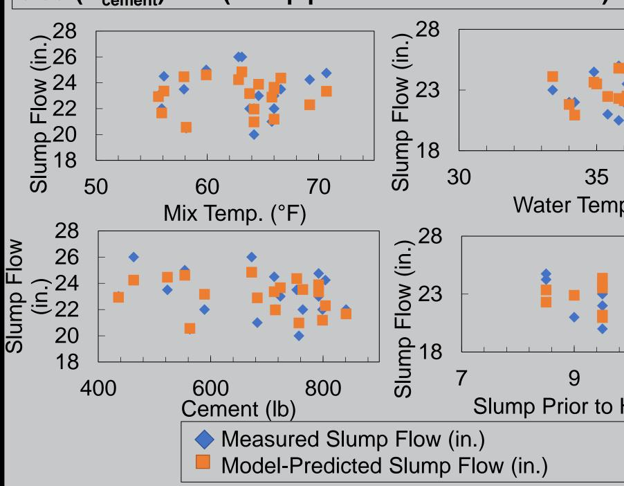
This model indicates that the most significant contributors to slump flow are mix temperature, water temperature, cement content, and slump prior to the addition of HRWR.
