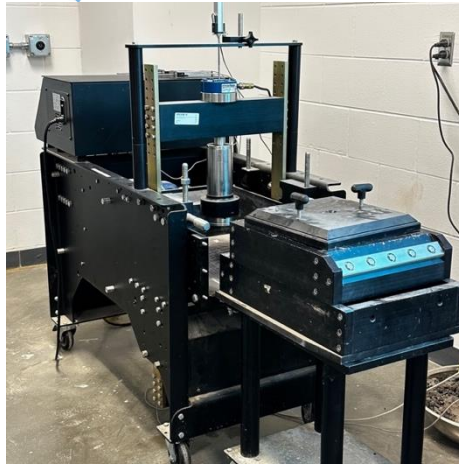
Figure 1: Large-scale direct shear test apparatus
