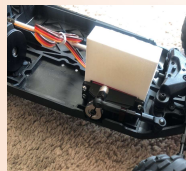
Fig 3: Installation of servo motor-arm, allowing to produce twice the torque as the original arm
