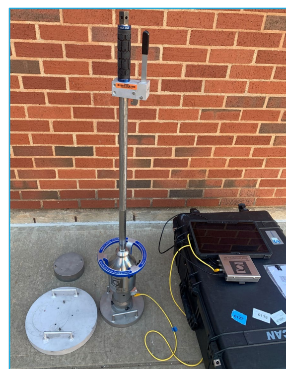
Deflection-Based Compaction Control
