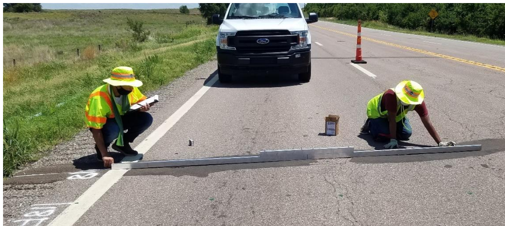
Figure 2.4 Photographic view of straightedge measurement in US-270
