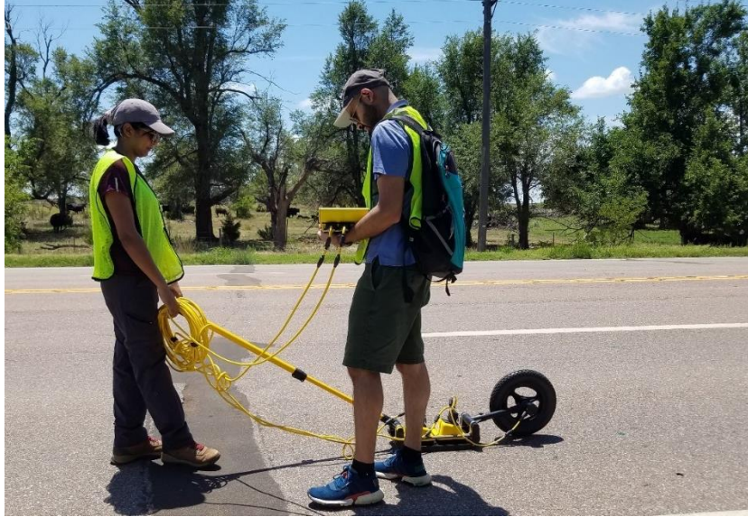
Figure 2.5 Photographic view of GPR testing in US-270
