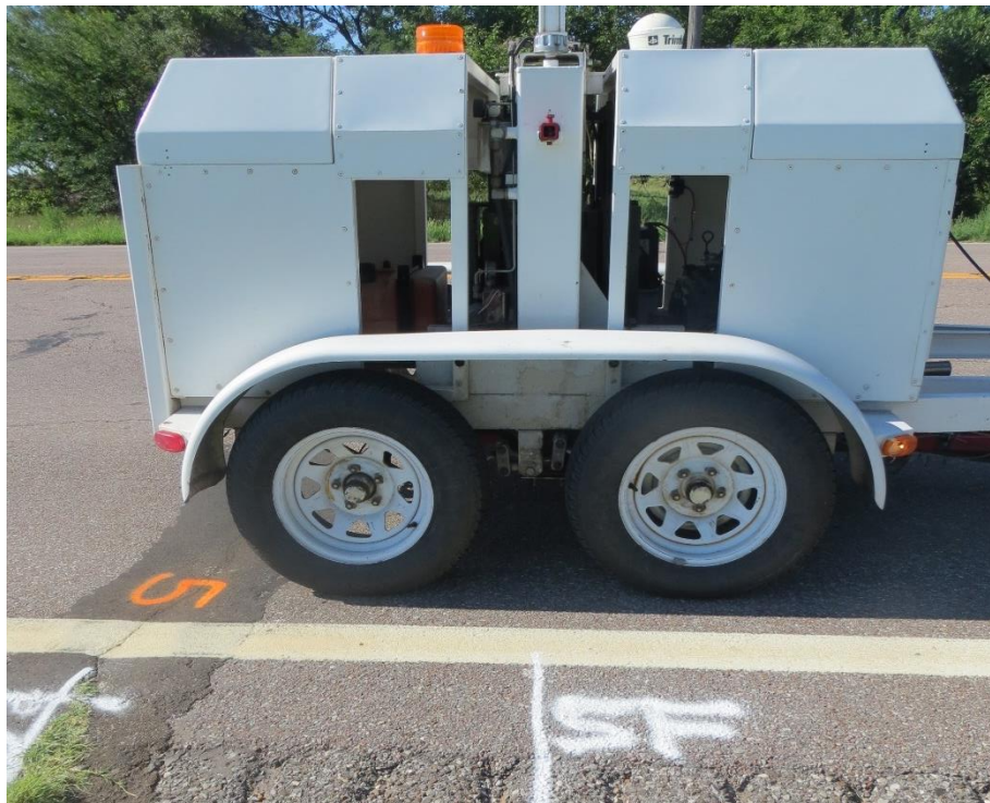
Figure 2.6 Photographic view of the FWD testing in US-270
