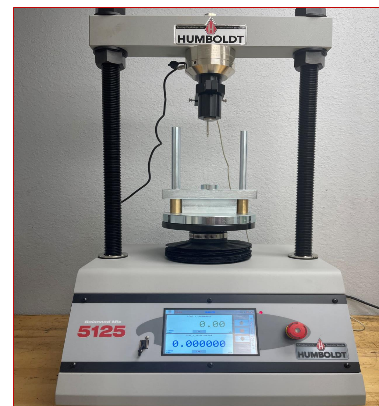
Figure 5. Testing Load Frame AASHTO T283
