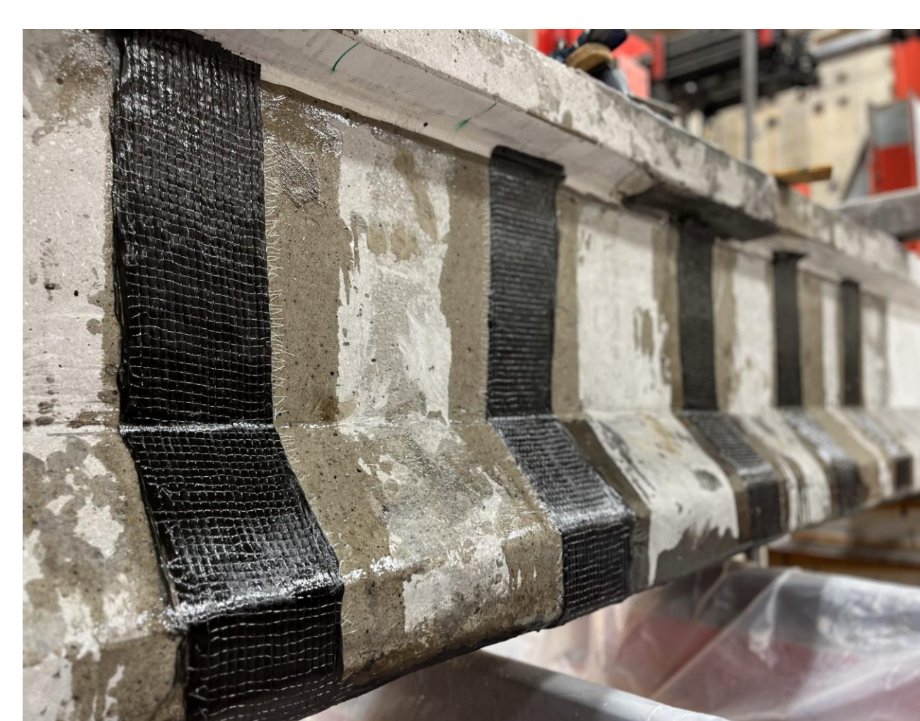
Longitudinal and transverse CFRP wraps
