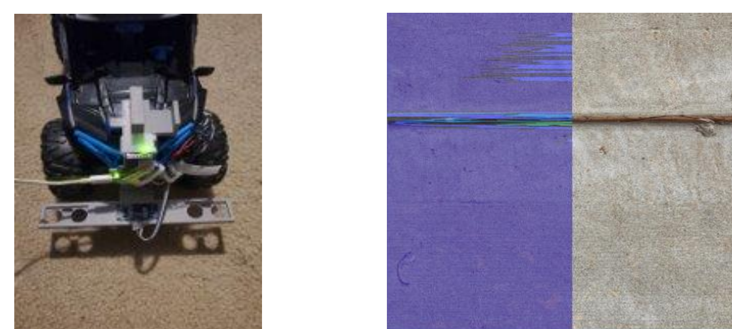
Figure 3 - (Left) First attempts for data collection using a single HC-SR04, Arduino Nano Every, and an MPU-6050 Accelerometer attached by a 3D-printed mounting device to a toy rover truck. (Right) First successful image from testing showing a contour plot overlaid (left-half) on the crack it detected, concrete spacers were a good starting point since a standard distance is used and can be measured and referenced easily.
