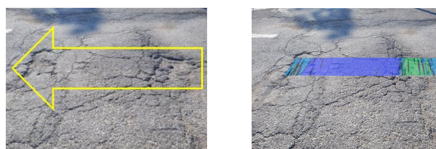
Figure 4 - (Left) Pothole 1 with area and direction scanned indicated with yellow arrow. (Right) Pothole 1 with contour map overlay.
