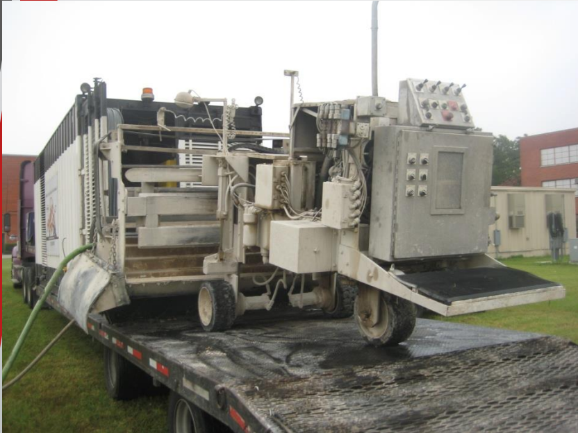
Hydro-demolition Robot on Truck Bed
