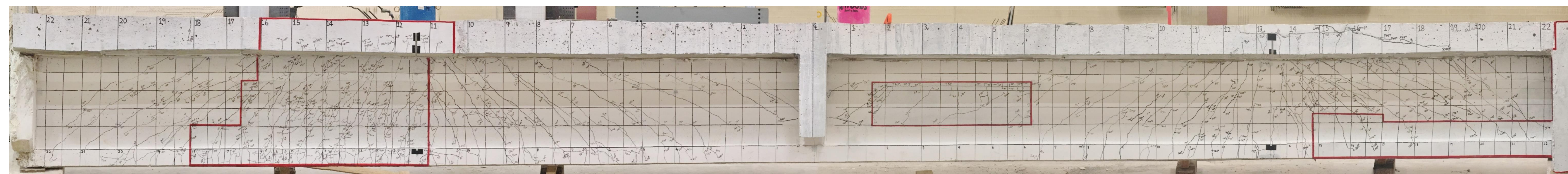
West Elevation of Resulting Damage from Initial Testing (Above) & Resulting Damage from Repair Testing (Below)
