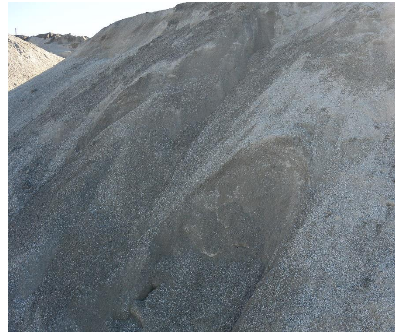
Fine Stockpile % Moisture \approx 3 to 7%
