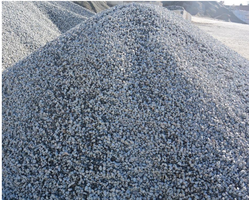
Coarse Stockpile % Moisture \approx 0.5 to 2%
