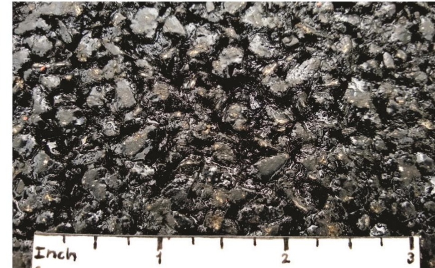
FIGURE 1 – Coarse Surface Texture of TOM.
