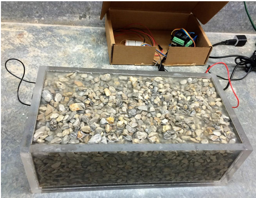
Figure 14: Fully Saturated AASHTO No. 57 Gradation of RE Janes Material Sample connected to INA219 Device
