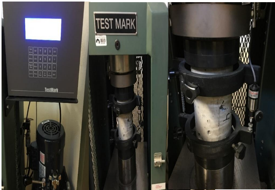
Figure 4.4. Pictorial View of Elastic Modulus Testing
