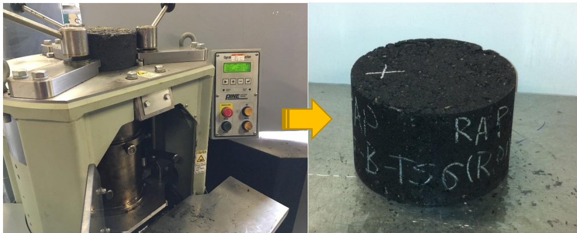
Figure 3.7 ITS Sample preparation
