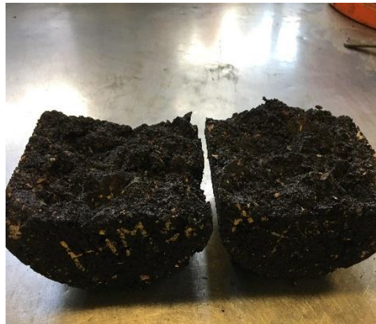
Figure 3.16 ITS Sample After Testing
