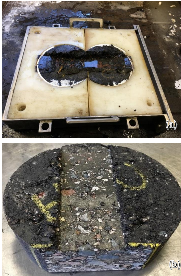
Figure 3.19 HWT Samples After Testing: (a) Severe moisture-induced damage; and (b) Minimum Moisture-Induced Damage
