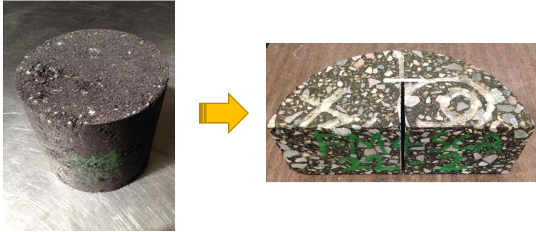
Figure 3.8 SCB Sample Preparation
