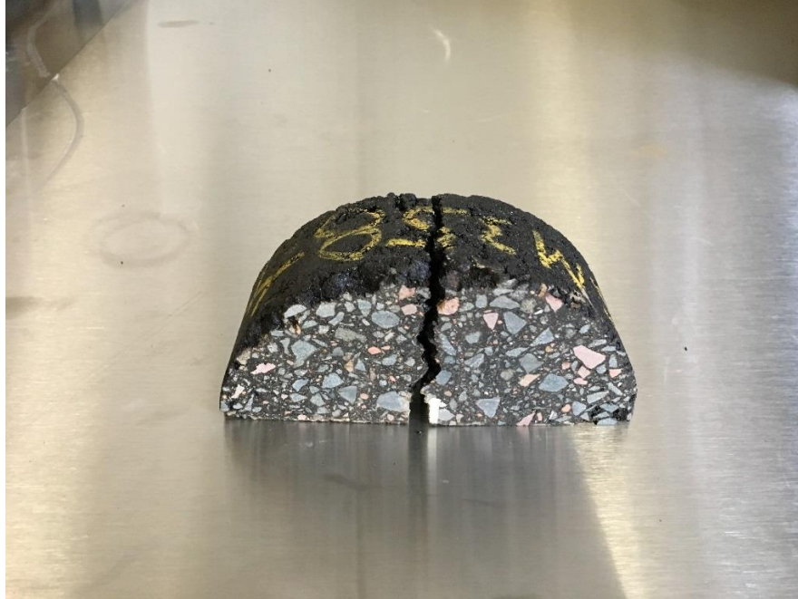
Figure 3.12 SCB Sample After Testing
