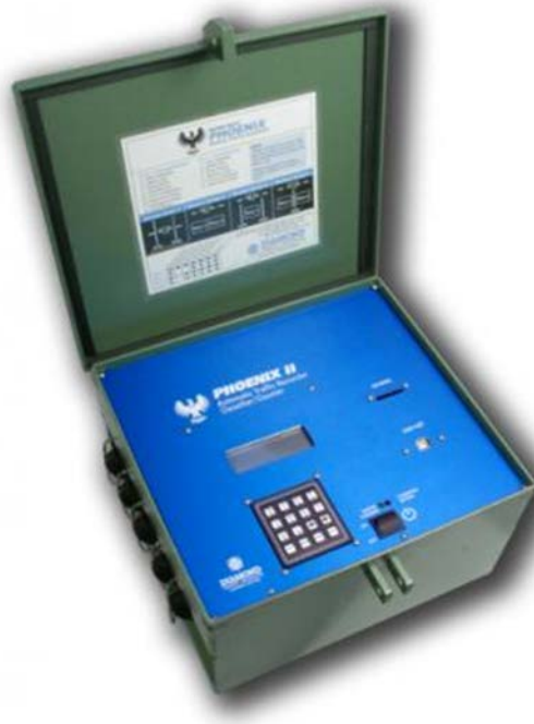
Figure 3-22 Phoenix II Diamond Traffic Unit.
