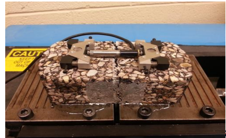
Typical cracking failure on OT specimen
