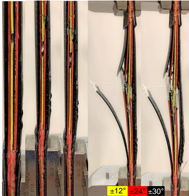
New FRP with Progressive sequential Drops
