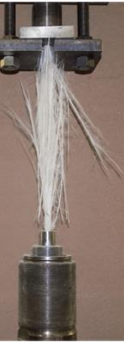
Pultruded GFRP with Brittle failure
