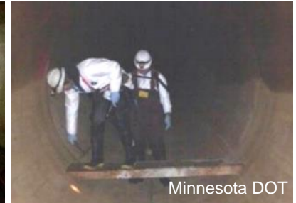
Minnesota DOT Hammer sound test
