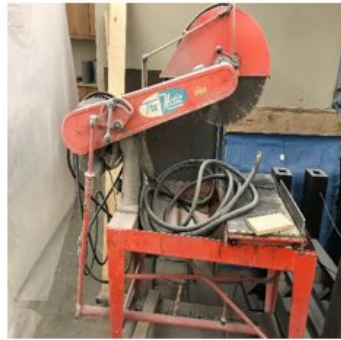
Saw used to prepare semicircular specimens
