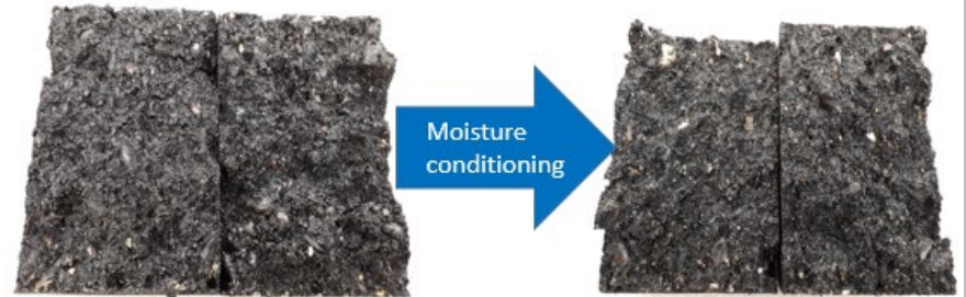
Failure surface of the dry sample and moisture-conditioned sample
